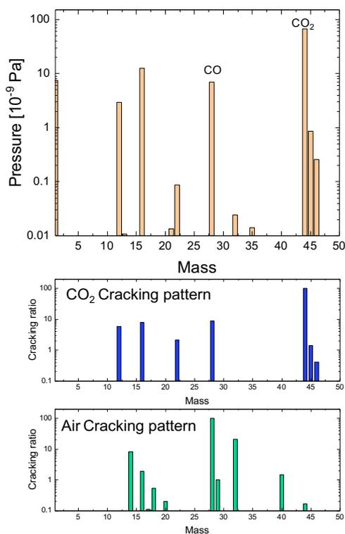
Fig. 1 Mass spectrum for gas in reaction chamber after Li-CO<sub>2</sub> reaction test
