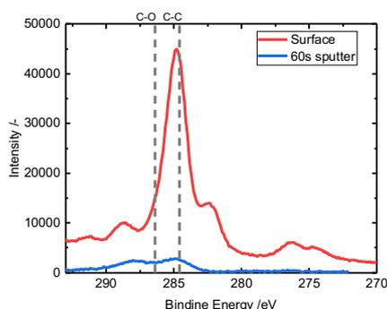
Fig. 2 XPS spectra of C 1s for SS-316.
