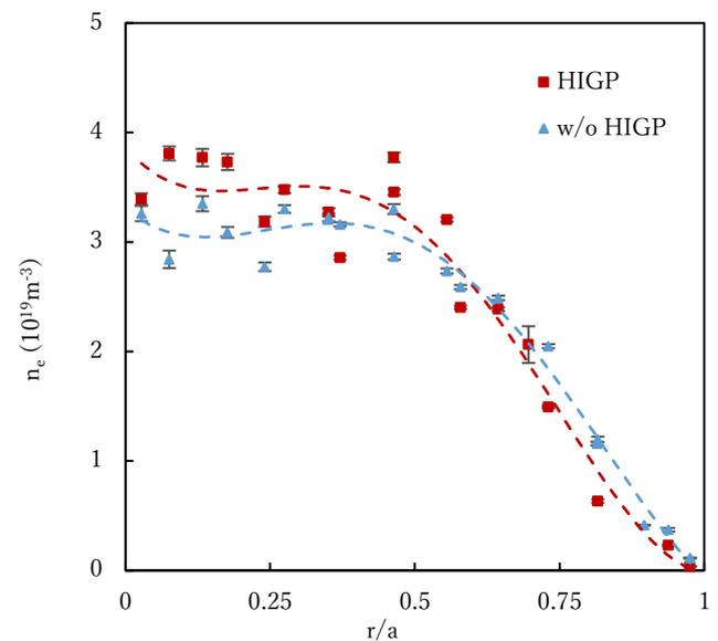
Fig. 2 Electron density profile with and w/o HIGP
