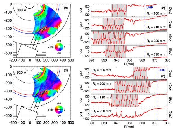
Fig. 2: Comparison of 2-D and 1-D wave pattern of phase for different toroidal magnetic field.
