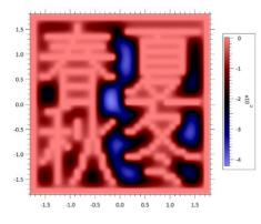
Keeping the conditions of F(x) and G(x) all over the domain, this solver can be also applied only to a part of the domain for calculating the potential u(x)in the part, as shown in the following figure. The development of the solver is successfully in progress.
