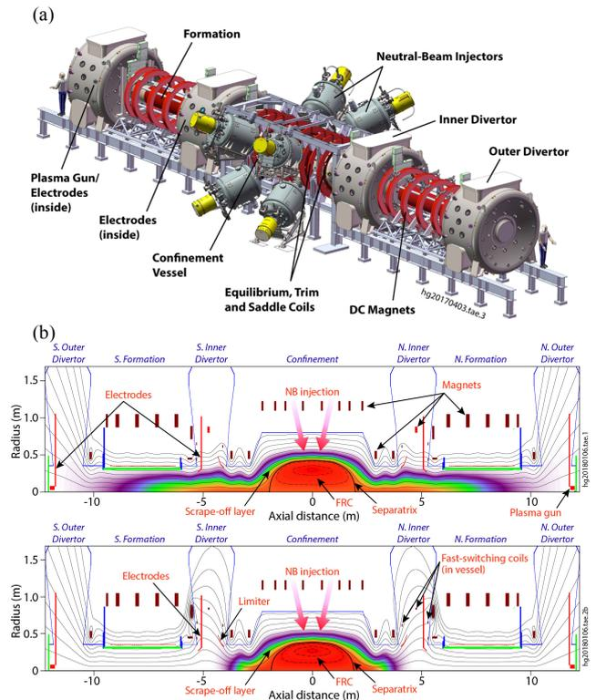
FIG. 1. (a) C-2W experimental device, “Norman”; (b) Sketches of FRC magnetic topology and density contours in 2 different operating regimes (edge biasing using outer divertors or switched to inner divertors), simulated by the 2-D MHD LamyRidge equilibrium code.
