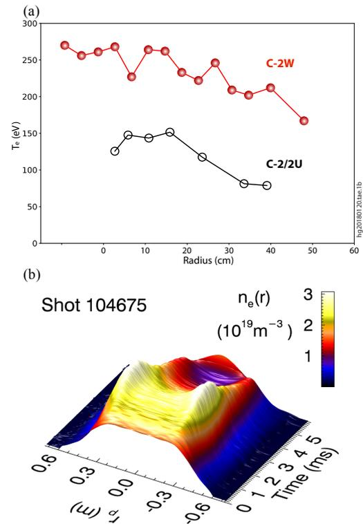
FIG. 2. (a) Electron temperature profiles at right after FRC collision/merging ( $t \sim 0.05$  ms) obtained in C-2/2U and C-2W; (b) density profile time evolution in C-2W. Both Thomson scattering and interferometer systems are located in the device midplane.
