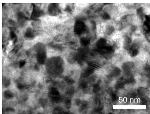
Fig. 1 Cross-sectional TEM image of  $Fe^{3+}/He^+$  irradiated/implanted  $Y_2O_3$  coating.
