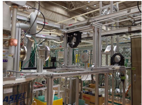
Fig. 1 303 GHz gyrotron (left hand side) and mirrors for coupling of the 303 GHz beam to the 3.5 inch corrugated waveguide system.
