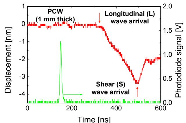
**Fig. 1:** Surface displacement at the epicenter measured at the back surface of PCW sample.
