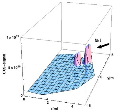
Fig. 3. Signal (two peaks) from He<sup>+</sup> ions excited by NBI and drifted He<sup>+</sup> plume ions.
