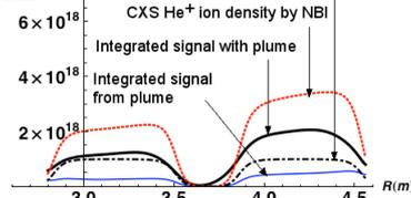
Fig.4. Integrated signal with He<sup>+</sup> plume along the viewing line for  $n(0)=1.0 \times 10^{19} \text{ m}^{-3}$  and  $T_e(0)=1.5 \text{ keV}$ .
