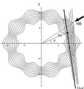
Fig. 1. 2D magnetic field line on the equatorial plane and the observing lines of the CXS in the LHD.
