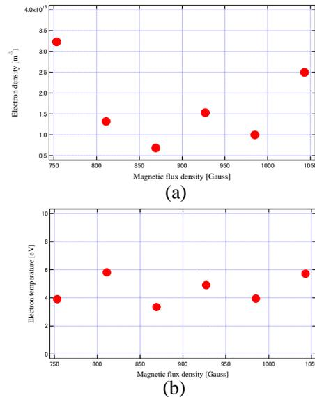
Fig.2 Coil current characteristics of electron density (a) and electron temperature (b)
