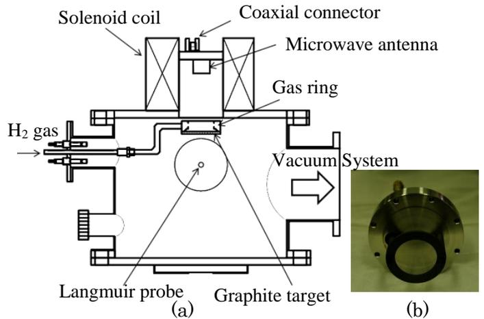
Fig.1 (a) Schematic diagram of ECR plasma apparatus. (b) Photograph of a carbon antenna with flange.
