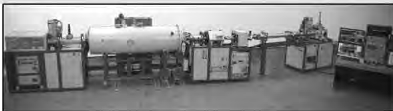
Pelletron Model 3SDH equipped with the NEC RF Charge Exchange Ion Source for H^+ and He^+ production and the Model RC43 analysis endstation
