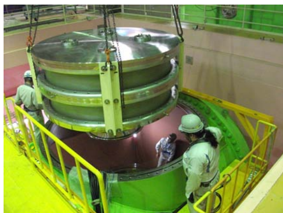
Fig.2 Full-scale two-stage mockup bushing
