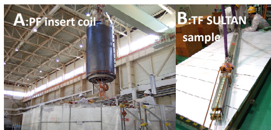
Figure 2 PF insert coil and TFC SULTAN sample.
