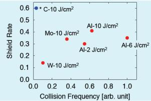
Fig. 4. Shield rate vs. collision frequency Target materials are Aluminum, Carbon, Mlybdenum, and Tungsten. The number/cm<sup>2</sup> indicates the laser energy density.
