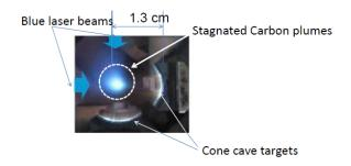
Fig. 1 Experimental Configuration Two soli targets with cone cave shape are irradiated with two blue laser beams. The ablated plumes cross each other at 1.3 cm.
