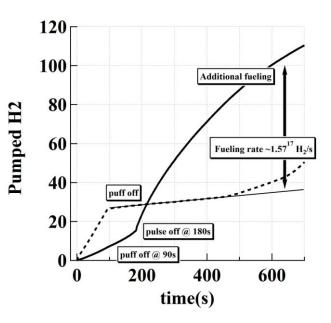
*Fig. 2 Global gas balance for #19674(180s discharge). The puff was stopped at 90 sec.*
