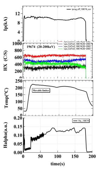
Fig. 1 Time evolution of SST plasma; (a) Ip, (b) HX (co-red, vertical-blue, vertical-green, ctr-black), (c) temerature of the movable limiter, (d) Hα from the CS region.
