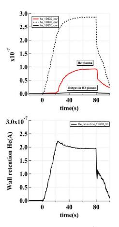
Fig. 3 Global gas balance for #19637(20s duration). The He puff was done during the pulse. All valves are closed.
