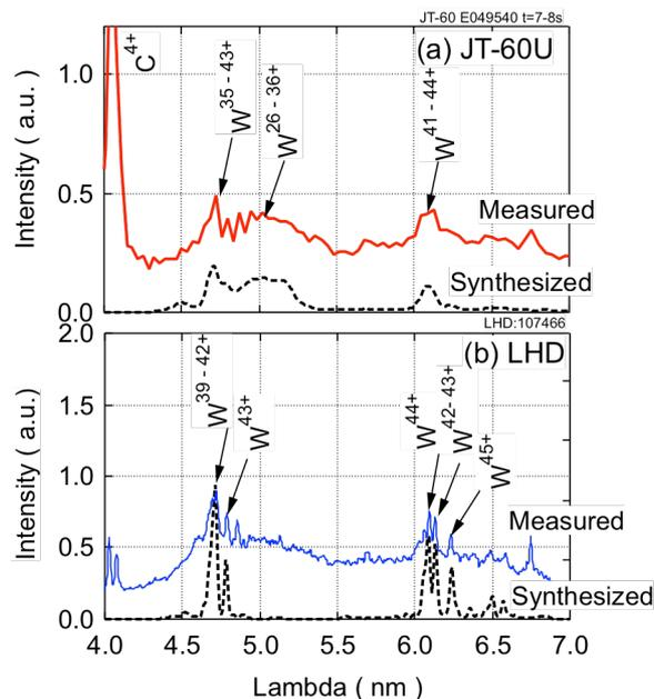
Fig. 1. Measured and synthesized spectrum (a) for JT-60U and (b) LHD.
