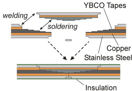
Fig. 3. Bridge-type joint of the REBCO conductor.
