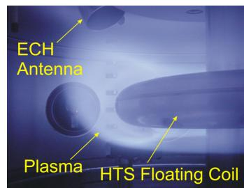
Fig. 5. The levitated Mini-RT HTS coil (present).
