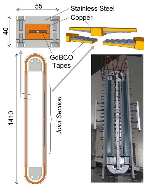
Fig. 4. The 30-kA class GdBCO conductor sample.
