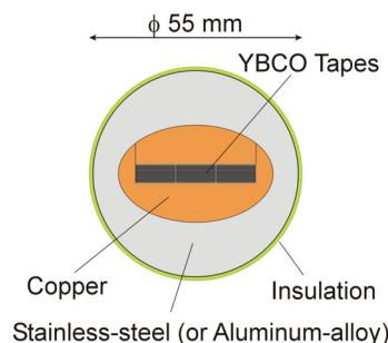
Fig. 1. A 100-kA HTS conductor design for FFHR-d1.
