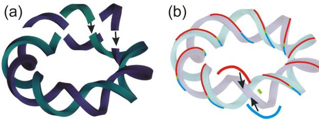
Fig. 2. Comparison between (a) joint of “coil-segments” and (b) “conductor-segments”.
