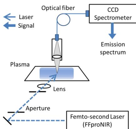
Fig. 1. Schematic diagram of the optical system measurement
