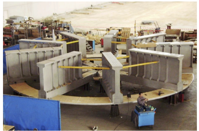
Fig.6 Pre-assembly of lower structure for cryostat base
