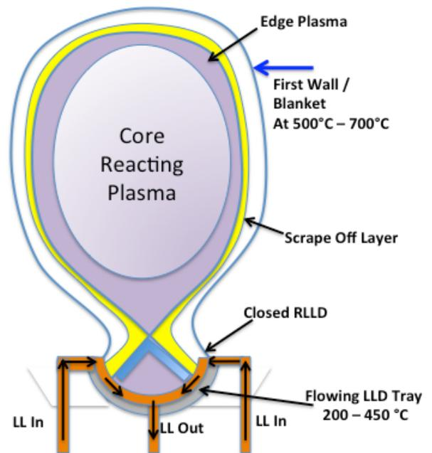
Fig.1. A possible RLLD configuration in a fusion power plant.
