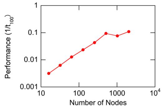
Fig. 1 Strong scaling of MEGA code vs. number of nodes on Helios.
