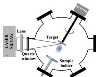
Figure 1. Schematic representation of the Nd:YAG PLD experimental setup
