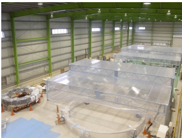
Fig.4 Fabrication of EF coils in Naka
