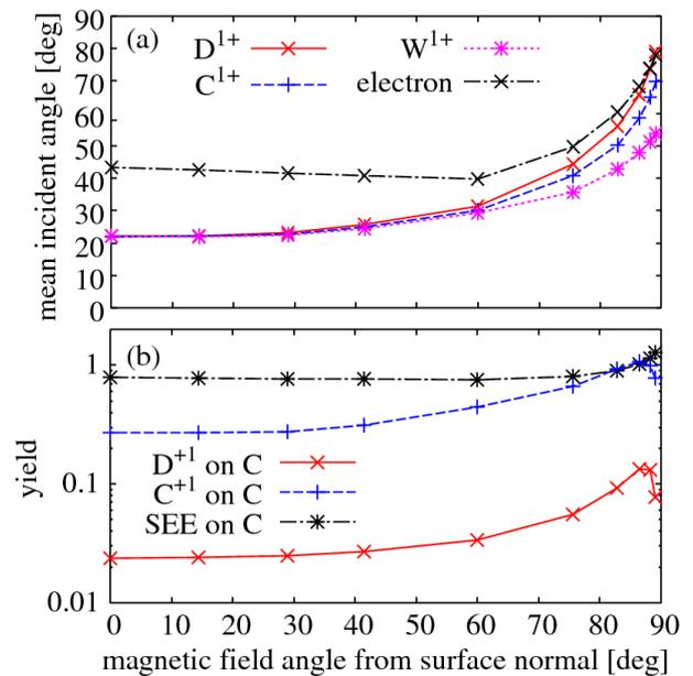
Fig. 1: (a) Incident angle distributions and (b) sputtering and secondary electron emission (SEE) yields obtained for various angles of the uniform magnetic field. The surface material is carbon.
