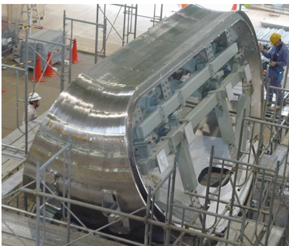
Fig.5 Assembly of VV 40-degree sector in Naka
