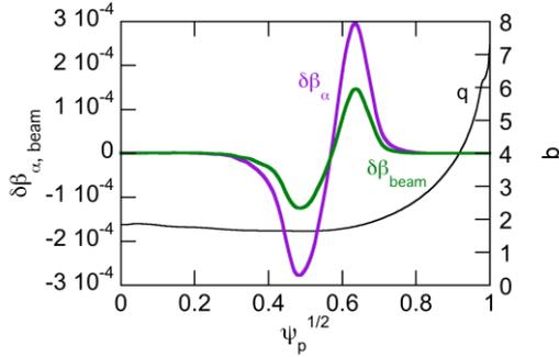
Fig. 3 Beta value perturbations for energetic alpha particles and beam deuterium particles, and safety factor profile.
