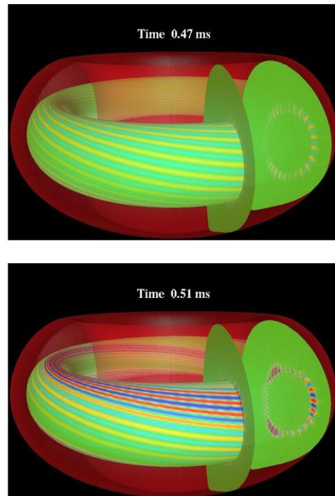
Fig. 2 Spatial profiles of TAE modes in the linearly growing phase (top) and in the saturation phase (bottom).
