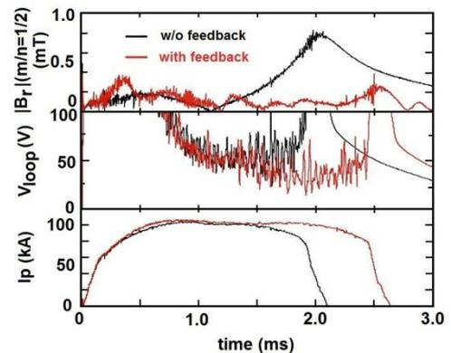
Fig.2: Effect of feedback control of the  $m=1/n=2$  mode on plasma performance.
