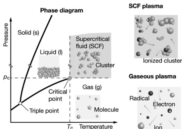
**Fig.1 Supercritical fluid (SCF) & SCF Plasma**
