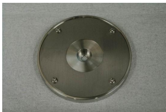
Fig.3 Holder for a glass plate sample.
