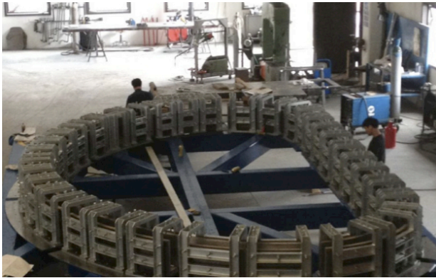
Fig. 3 Impregnation mould of winding pack TF coil
