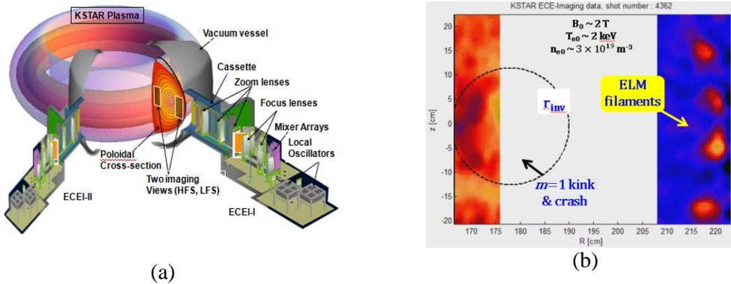
Fig.1 (a) Two toroidally separated ECEI systems on KSTAR. ECEI-I has two independent views that are capable of measuring two views simultaneously. ECEI-II has a single view of ECEI and MIR system to measure 2D density fluctuations. (b) Simultaneous measurement of the core  $m=1$  mode and edge localized mode (ELM) by the ECEI-II system.
