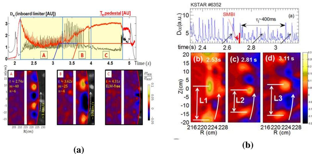
Fig.2 (a) The time evolution of the ELM during RMP experiment. Upper time traces:  $D_\alpha$  signal and edge  $T_e$ . (A)-Image of the ELM before the RMP power is applied, (B)-intensified ELM image during RMP phase, (C)-Image during the suppression phase of the ELM. (b) The time evolution of the ELM during SMBI experiment. (b)  $D_\alpha$  signal (a) Image of the ELM prior to the SMBI (b) EM structure during the SMBI (c) Recovery phase of the ELM (d)
