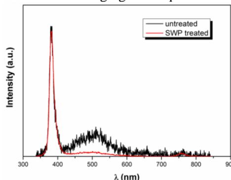
Figure 2. PL measurements of ZnO obtained by PLD and SWP treated.
