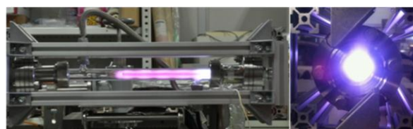
Figure.1 Structure and picture of the MIP light source. Upper one: structure Left one: side view; Right one: front view.
