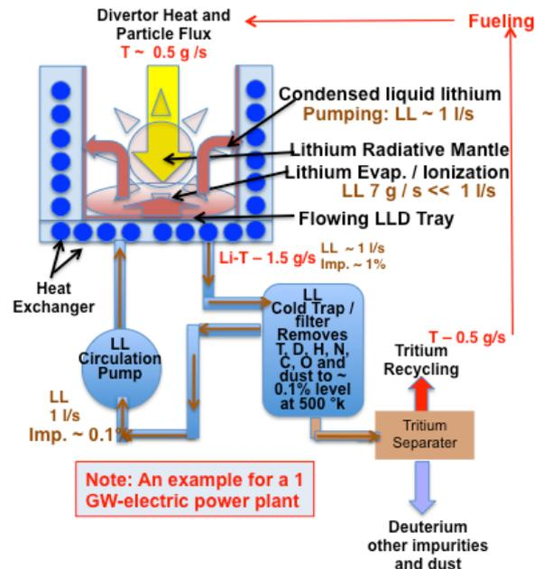
Fig.3. A schematic for the RLLD purification loop.
