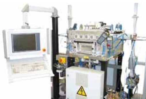
Picture of the eight-linear antenna type micro-wave plasma CVD equipment.
