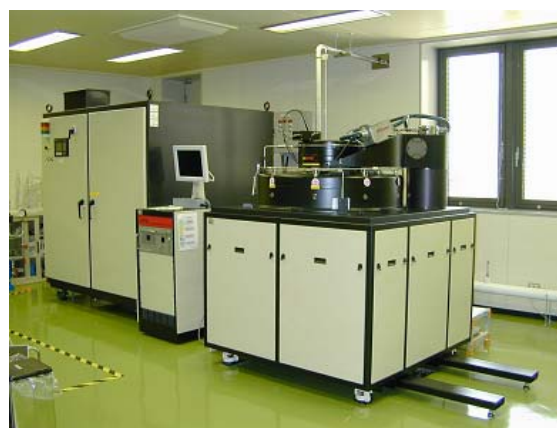
Fig. 1. 915-MHz microwave plasma CVD reactor for diamond film synthesis. It can coat a film over a 6-inch substrate.
