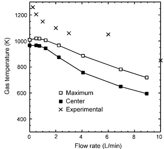
Fig. 4 Maximum and central gas temperatures as a function of the forced gas flow rate for He ( $=0.5 \text{ MW/cm}^3$ ), together with experimental values for  $\text{He/N}_2(5\%)$  discharge at a microwave power of 100W.
