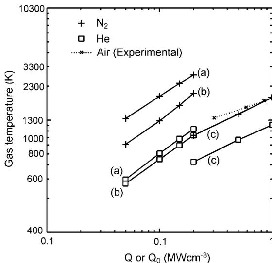
Fig. 3 Gas temperature at the center of the heating zone as a function of  $Q$  or  $Q_0$  for He and  $\text{N}_2$  gas in cases of (a) static gas, (b) flowing gas with  $Q=\text{constant}$ , and (c) flowing gas with  $Q=Q_0 n_g/n_0$ . Experimental results for air discharge in the microwave power range of  $\sim 30\sim 100\text{W}$  are also shown, where the horizontal position of the plot is arbitrary chosen.
