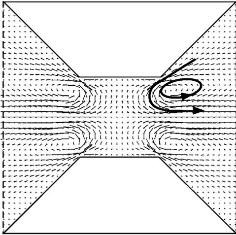
Fig. 2 Flow vector diagram in the central part of the simulation space for He without forced gas flow ( $Q_0 = 0.5 \text{ MW/cm}^3$ ).
