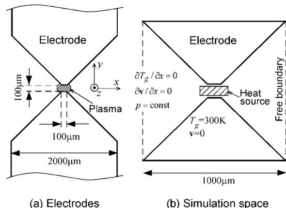
Fig. 1 Microgap discharge configuration and the simulation space for heat transport study.
