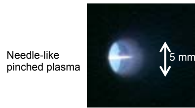
Fig. 2 Still photograph of the Z-pinch EUV plasma. View from 30^\circ for the z axis. The diameter of the discharge tube is 5 mm \phi .
