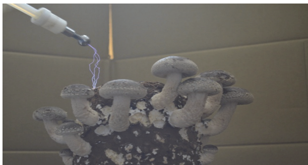
Fig. 3. Photographic image of discharge from high-voltage electrode to the sawdust-bed for L. edodes cultivation.
