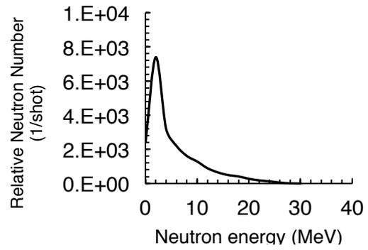
Fig. 4. Neutron energy spectrum
