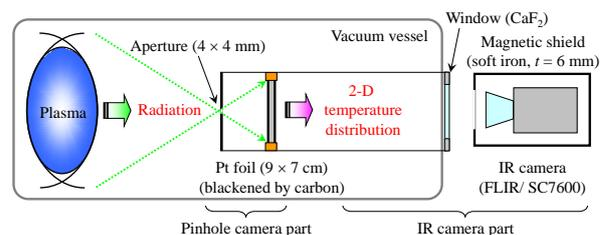
Fig.1. Schematic of IRVB
