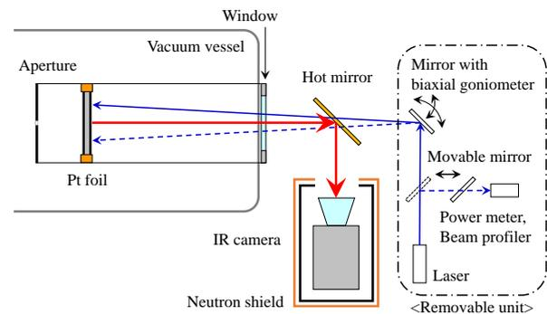
Fig.2. Schematic of in-situ calibration system for IRVB.
