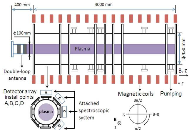
Fig.1 Schematic view of PANTA and the disposition of spectroscopic system
