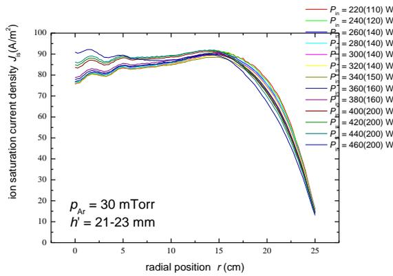
Fig. 2(a). Plasma distribution in the Antenna Type I.
