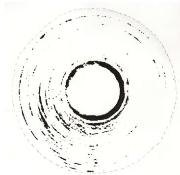
Fig.4 Burn pattern of 300 GHz Gyrotron Output Power.
