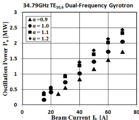
Fig.3 Calculated beam current dependences of 34.8 GHz TE<sub>10,6</sub> mode oscillation powers.
