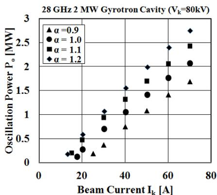
Fig.2 Calculated beam current dependences of 28GHz TE<sub>8,5</sub> mode oscillation powers .
