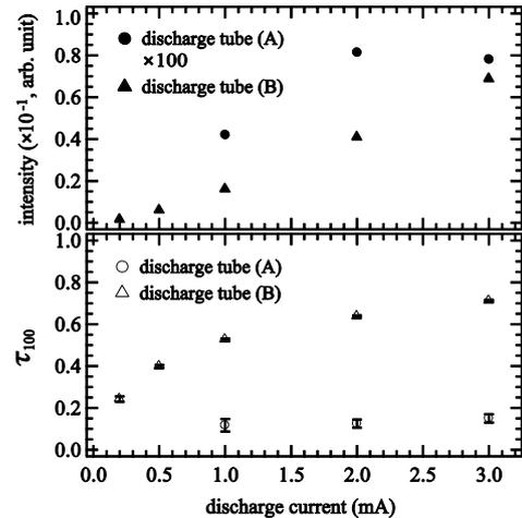
Figure 2. Observed variations in the total emission intensity and  $\tau_{100}$  as a function of the discharge current.
