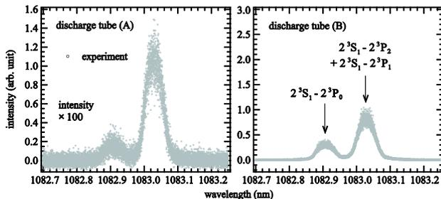
Figure 1. HeI  $2^3S$ - $2^3P$  spectra observed in the discharge tubes (A) and (B) at a discharge current of 3 mA.
