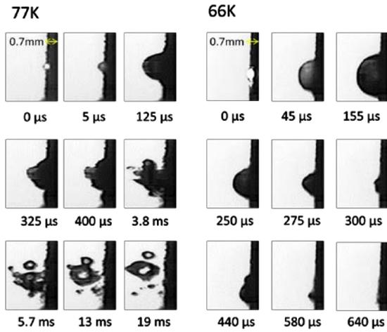
Fig. 2 Pictures of cavitation bubbles observed in liquid nitrogen at temperatures of 77 and 66 K. The pressure was 0.1 MPa.
