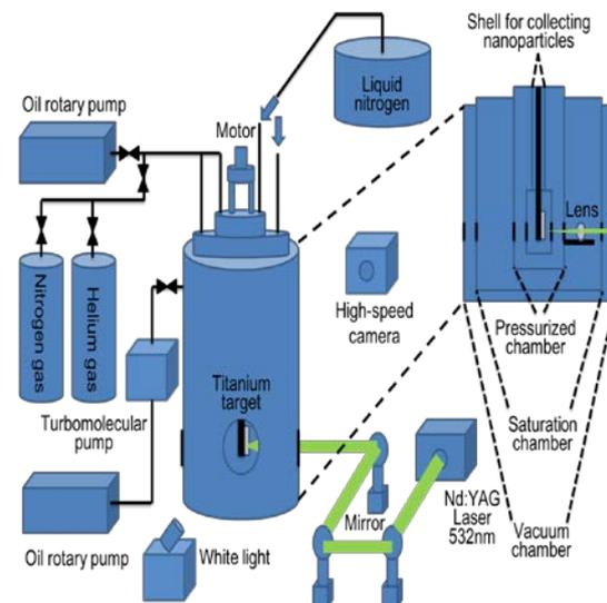
Fig. 1 Experimental apparatus for laser ablation in liquid nitrogen at an arbitrary temperature between the freezing and boiling points.
