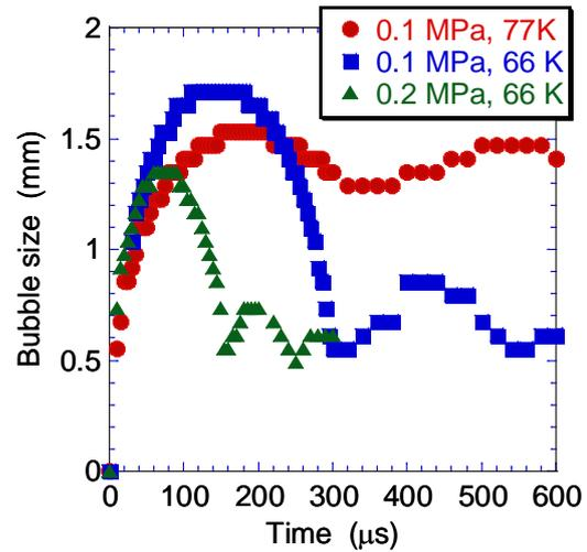
Fig.3 Temporal variation of the bubble size observed at different temperatures and pressures.
