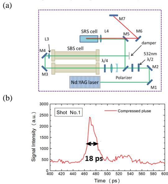
Fig.2 (a) Setup of a 20 ps probe laser pulse generation utilizing SBS and SRS pulse compression schemes. Laser pulse with 532 nm of wavelength and 7 ns of duration is compressed down to 300 ps in the SBS cell. The 300 ps pulse is compressed again down to 20 ps in the SRS cell. Wavelength of the laser is changed to 630 nm by the Raman scattering. (b) Temporal profile of the compressed pulse.
