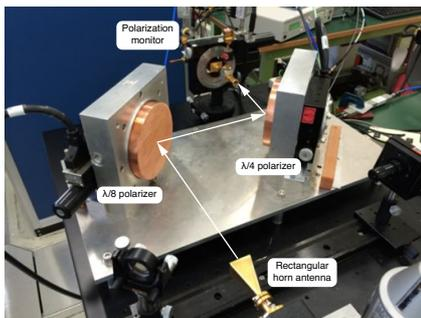
Fig. 1. Low power test setup. The polarization monitor with a fast digitizer with an FPGA is newly installed.
