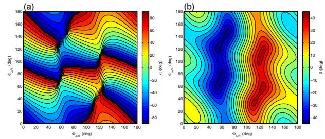
Fig. 2. Dependence of polarization parameters (a)  $\alpha$  and (b)  $\beta$  on the polarizer rotation angles  $\Phi_{\lambda/8}$  and  $\Phi_{\lambda/4}$  of the manufactured polarizers.
