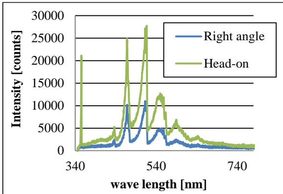
**Fig.2.** Spectroscopic measurement result of two arrangements; right angle and head-on collision.
