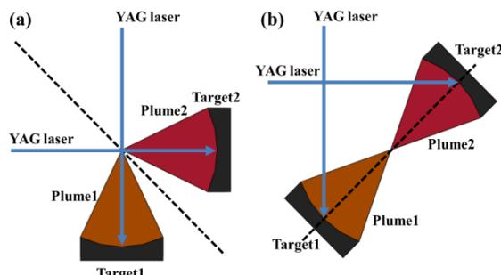
**Fig.1.** LEAF-CAP setup [2] (a) Right angle collision (b) Head-on collision
