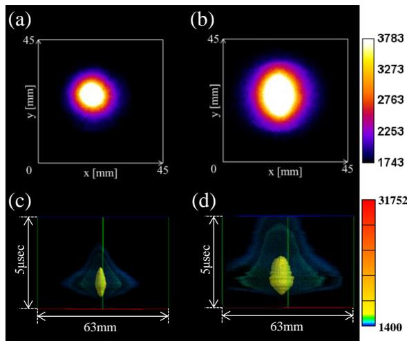
**Fig.3.** ICCD images 1.2  $\mu$ sec after the beam irradiation, (a) Right angle collision (b) Head-on collision. Spatial integrated images, (c) Right angle collision (d) Head-on collision.
