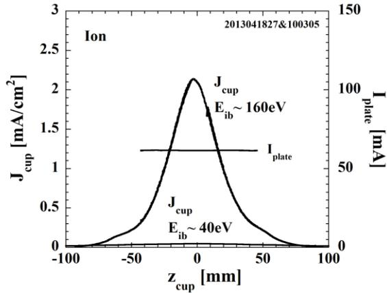
Fig.2 Profiles of ion beams with different  $E_{ib}$ , 40 and 160 eV.
