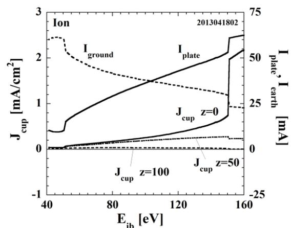
Fig.1 Variations of current densities,  $J_{\text{cup}}$  at the beam center ( $z=0$ ), at  $z=50\text{mm}$  and  $100\text{mm}$ , and,  $I_{\text{plate}}$  and  $I_{\text{ground}}$  as functions of ion beam energy,  $E_{\text{ib}}$ .
