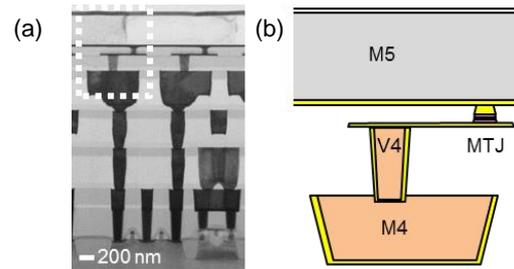
Figure 2 (a) Cross sectional TEM photograph of the spintronic devices with MTJ, and (b) enlarged schematic illustration of the part indicated by the rectangular dot on (a) [8].
