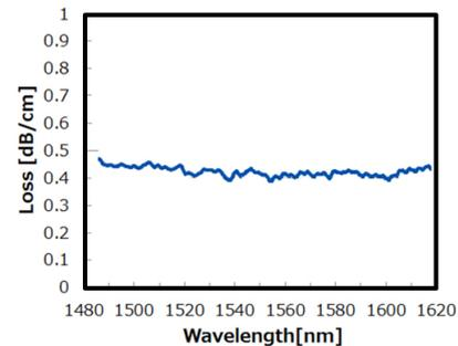
Figure 4 Propagation loss of TE mode as a function of wavelength [12]. The Si-WG was fabricated with using an immersion-ArF lithography technique.
