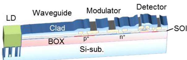
Figure 1 Cross sectional drawing of a typical silicon photonic device [12]. It is fabricated with using specially designed SOI wafer for the silicon photonics. Actual device includes high-speed RF electrical wiring (not shown here) to handle information electrically. Embedding many types of elements into one chip is one of the characteristics of this device.
