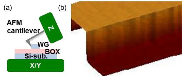
Figure 3 (a) Schematic illustration of 3D-AFM system, and (b) 3D-AFM image of Si-WG [11].
