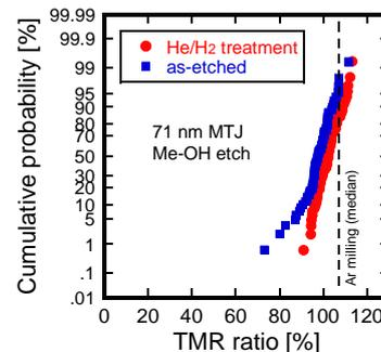
Figure 6 TMR ratio distributions of the 71 nm MTJ over the as-etched and the He/H<sub>2</sub>-plasma-treated 300 mm wafers [18]. Median TMR ratio obtained from a small sample fabricated with Ar milling is also indicated by the broken line.
