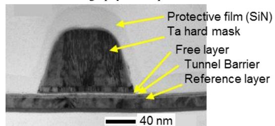
Figure 5 Cross sectional TEM image of a MTJ etched by Ar/NH<sub>3</sub>/CO gas system [16].
