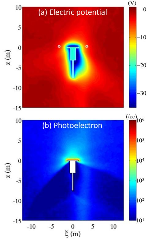
Fig.2. 2-dimensional profiles of (a) electric potential, and (b) photoelectron density
