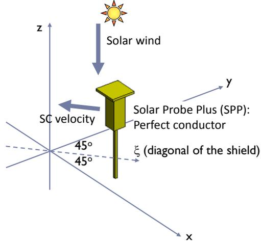
Fig.1. Model of Solar Probe Plus with simplified geometry
