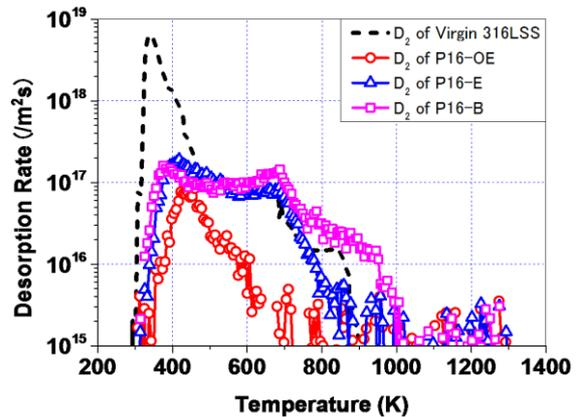
Fig.2 TDS spectrum of D<sub>2</sub>
