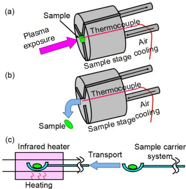
Fig. 3. Schematics illustrating the processes to transport a sample from the plasma irradiation region to the TDS measurement region.
