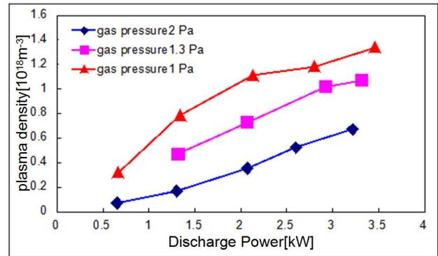
Fig. 4. Discharge power dependence of the deuterium plasma density.
