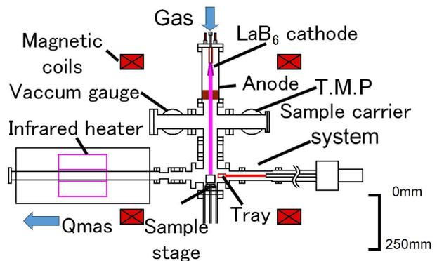
Fig. 1. A Schematic of the compact divertor plasma simulator (CDPS)
