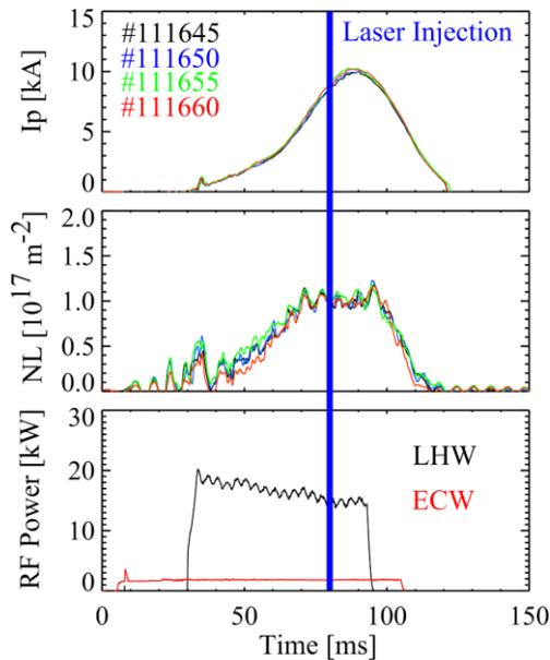
Fig.1. Typical waveforms in the present experiment. Blue line indicates the timing of laser injection at 80 ms.
