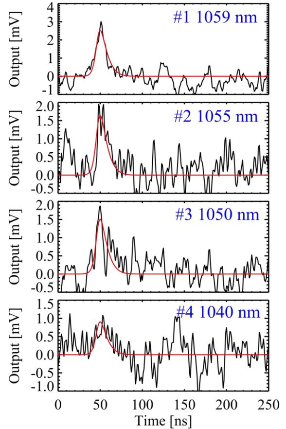
Fig.2. Background-subtracted TS signals detected in a polychromator at  $R \sim 389$  mm (black) and the pulse shape fitting (red). Each channel is sensitive around a wavelength (blue) written in each plot.
