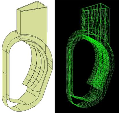
Fig.1 Example of conducting shells and vacuum vessel with maintenance port (left hand side) and (b) mesh model for eddy current analysis (right hand side)
