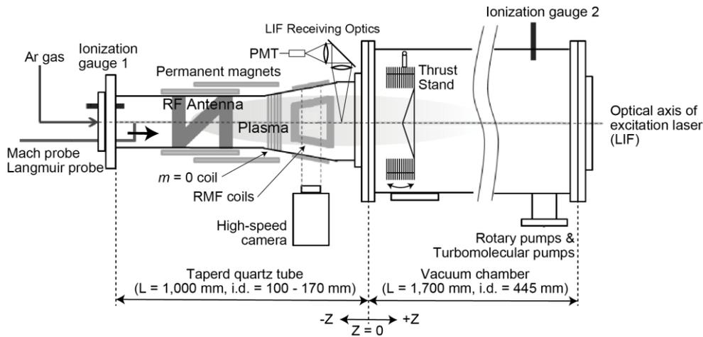
Fig. 1 Schematic diagram of large mirror device (LMD)
