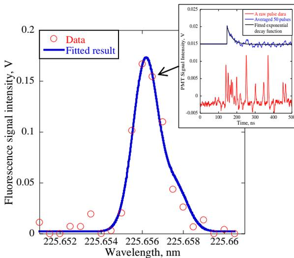
Fig. 3. Spectral data of two-photon absorption fluorescence from atomic oxygen & raw-analyzed pulse data
