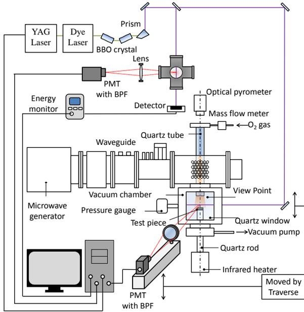
Fig. 2. Experimental setup of TALIF
