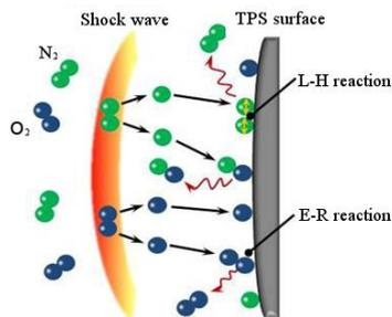
Fig. 1. Schematic of recombination model due to the surface catalysis on TPS surface.
