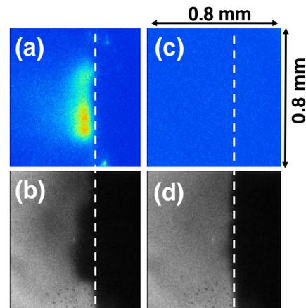
Fig.3. Images of optical emission of discharge ((a) and (c)) and shadowgraph of cavitation bubble ((b) and (d)). The phase difference between the group (a)/(b) and (c)/(d) was  $\pi$ .
