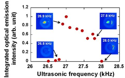
Fig.2. Relationship between the optical emission intensity of the discharge and the frequency of the ultrasonic wave.
