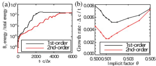
Fig.2. (a) Time evolutions of the magnetic energy for the first (black) and second (red) order shape functions. (b) Growth rate for different implicitness factors.
