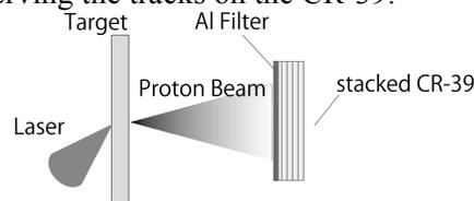
Fig.1. Schematic top view of the experimental setup. The “CR-39 stack” is set in the direction of the target normal.
