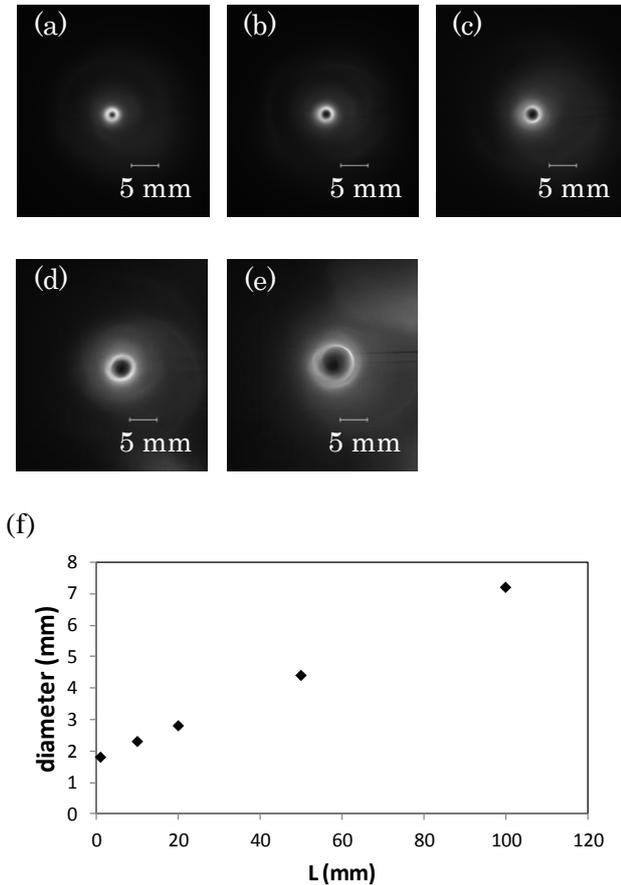
Fig. 2 (a), (b), (c), (d) and (e) Typical single-shot images of electrons emission obtained on the first layer IP with  $L = 1, 10, 20, 50$  and  $100$  mm. The color scale is set independently for maximum contrast. (f) The diameter of the ring as a function of  $L$ .
