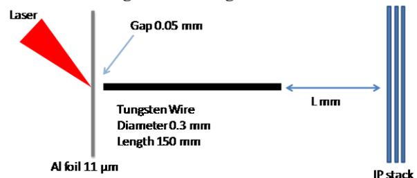
Fig. 1 Experimental setup to observe emitted electrons using stacked IPs.
