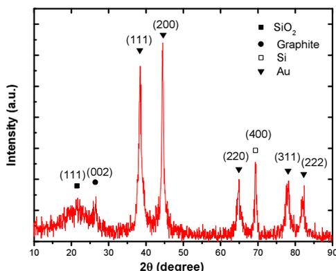
Fig. 2 XRD pattern of the graphite-encapsulated gold nanoparticles powder on Si substrate.
