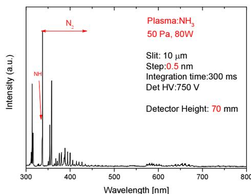
Fig. 3 Typical Optical emission spectra of the ammonia plasma generated by RF power of 80 W.
