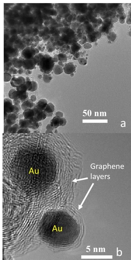
Fig. 1 Typical TEM image for the as-fabricated graphite-encapsulated gold nanoparticles. a) in smaller magnification, b) in bigger magnification
