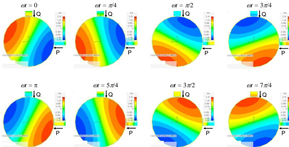
Fig. 5. Magnetic field profile on the plane  $z=0$  for successive wave phase ( $\omega t$ ).
