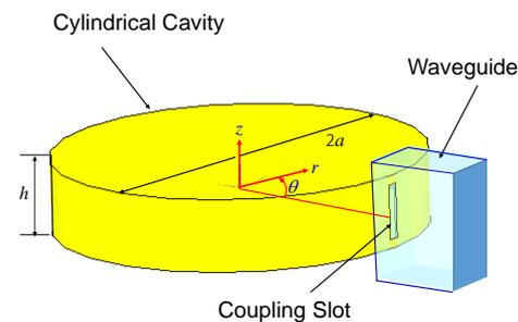
Fig. 1. Model of cylindrical cavity excitation.
