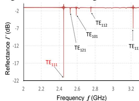
Fig. 2. Frequency spectrum of reflectance.
