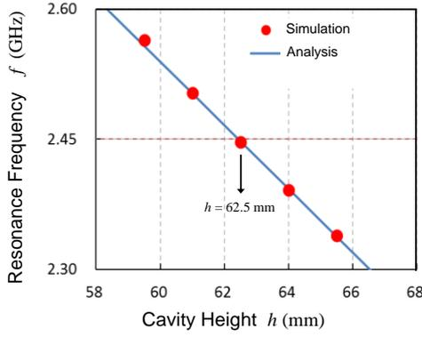
Fig. 3. Resonance frequency vs. cavity height.
