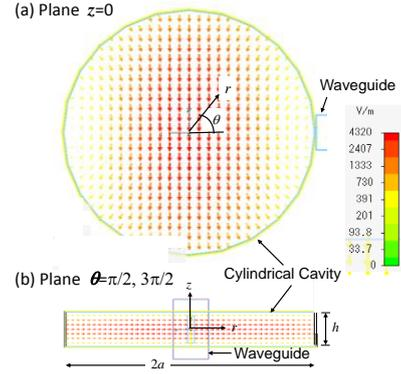
Fig. 4. Electric field vector distribution in cavity.
