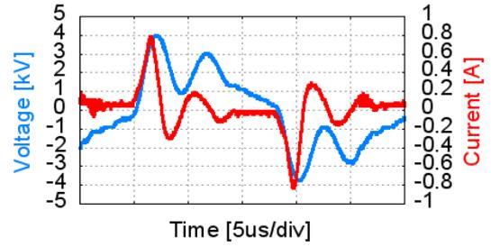
Fig.3. Typical time evolution of voltage and current waveforms in plasma jet reactor
