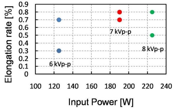
Fig.4. Relation between elongation rate and input power
