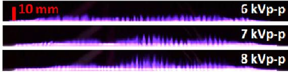
Fig.2. Photograph of the plasma jet at 100 L/min of flow rate of helium
