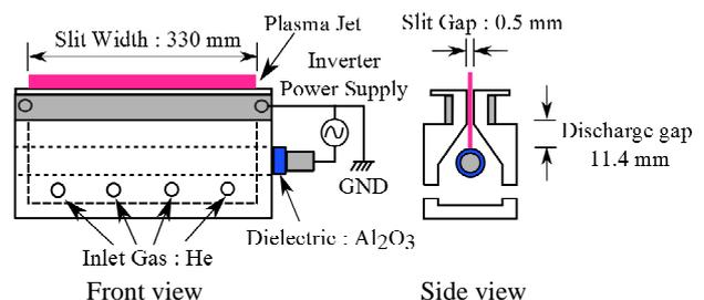
Fig.1. Conceptual diagram of the plasma jet reactor
