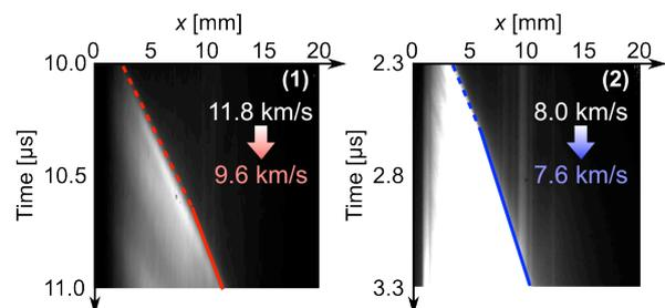
Fig. 2. Streak images of the plasma flow generated by the taper-cone-shaped plasma focus device.
