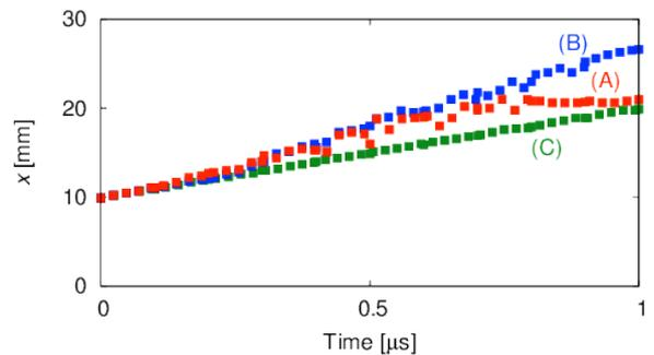
Fig. 5. Time evolution of the shock position calculated by the Hybrid PIC method.
